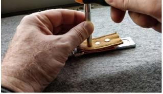
Check that the rivet is set. If the rivet has been set correctly you should be able to pick up the piece without the rivet stem or cap falling off. If they do fall off (or you feel you can move the rivet) reset them and give the setter a little bit of a harder bang.
