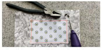
For that same reason, we are making the hole through the layers of fabric with an awl and not with a punch. The benefit of an awl is that you do not damage the fibers. You are only pushing them aside.
